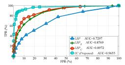
**Fig. 5.** ROC curves for binary classification of smoke and general non-smoke (*LBP*: extracted from the original image block  $\mathbf{f}$ ; *LBP*<sub>S</sub>: extracted from the quasi-smoke component  $\mathbf{D}_{s}\mathbf{y}_{s}$  only; *LBP*<sub>C</sub>: extracted from both the quasi-smoke component  $\mathbf{D}_{s}\mathbf{y}_{s}$  and the quasi-background component  $\mathbf{D}_{b}\mathbf{y}_{b}$  and then concatenated).
