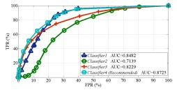
Fig. 7. ROC curves for single image smoke detection based on the four classifiers.
