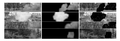
**Fig. 4.** Quasi-smoke and quasi-background separation (column 1: the test images, column 2: the separated quasi-smoke components, column 3: the separated quasi-background components).
